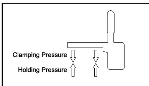
**ii) The clamping force** is the force that the clamp will exert on the component or work piece. It is dependent on the effort applied to the clamp (e.g. the length of the clamp handle or the strength of the operator). So values of clamping force given in Sandfield's literature are only guides based on what an average person can apply.
