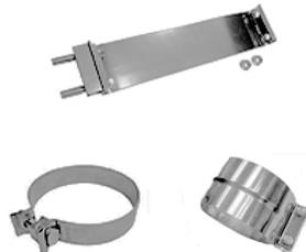
**Band Clamps:** "CI" and Torca® band clamps in preformed, flat and narrow band styles. Single bolt and double bolt installation. Size range from 1.75" to 6" depending on style.
